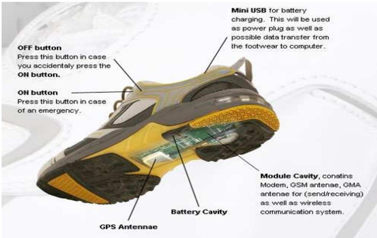
**Figure 11:** The GPS built into the heel of the shoes
